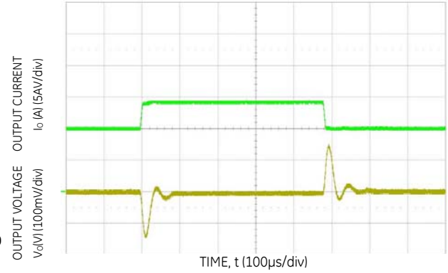
Figure 4. Transient Response to 1.0A/μs Dynamic Load Change from 50% to 75% to 50% of full load.
