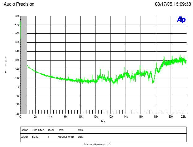
Figure 32 – Audible Noise V_{IN} = 230 VAC; I_{OUT} = 1.2 A.
