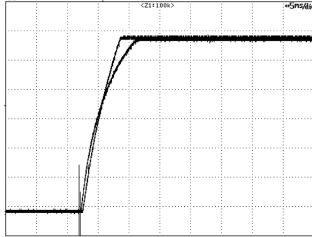
Figure 17 – Start-Up Profile, 230 VAC. Fast trace is no-load rise time. Slower trace is maximum load (12 \Omega ) 2 V, 5 ms / div.
