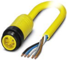
Power cable, 5-position, PVC, yellow, Plug straight 7/8"-16UNF, on free cable end, cable length: 2 m
