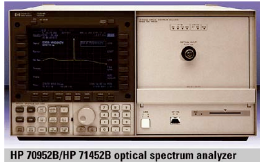
Photo 13. An optical spectrum analyzer is used to characterize the light outputs from LEDs and lasers.
