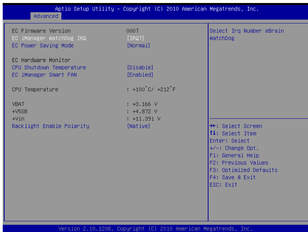
Figure 3.12 Embedded Controller Configuration
