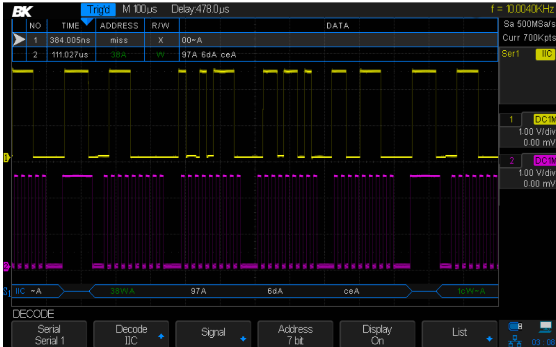
Figure 108 - I2C decode result
