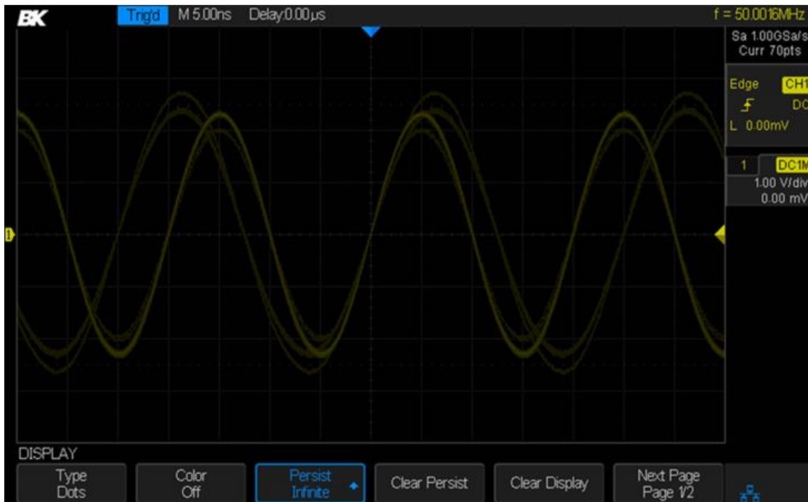
Figure 91 - Persistence set to infinite
