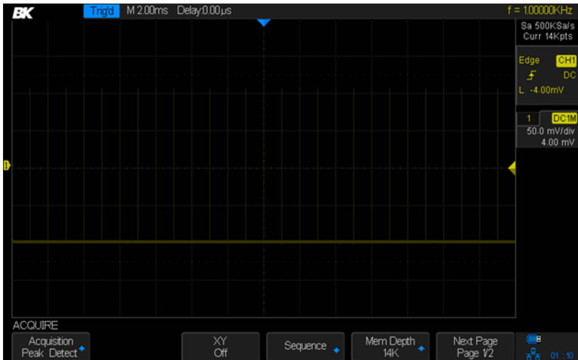
Figure 35- Pulse with 0.1% duty cycle, peak detect mode
