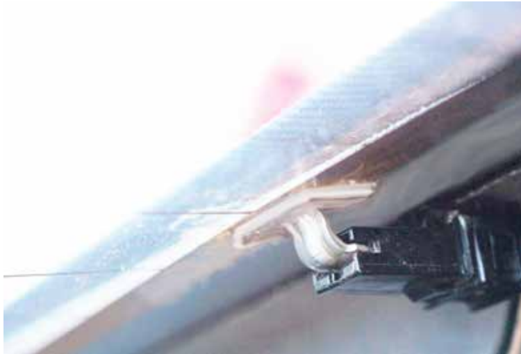
Very effective at bonding car rear defrost tabs back on the grid permanently.
