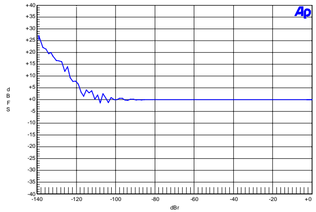
Figure 14. 96 kHz, Fade-to-Noise Linearity
