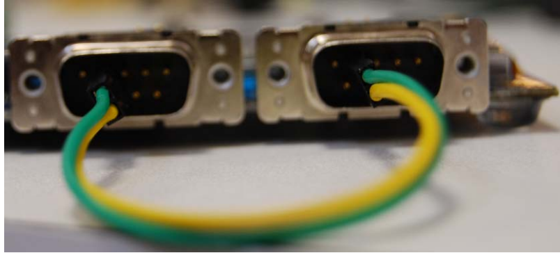
Figure 2-3. CAN loopback on the AT32UC3C-EK
