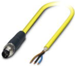
Sensor/Actuator cable, 3-position, PVC, yellow, shielded, Plug straight M8, on free cable end, Cable length: 10 m
