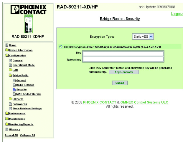
Figure 4-24 “Bridge Radio - Security” screen
